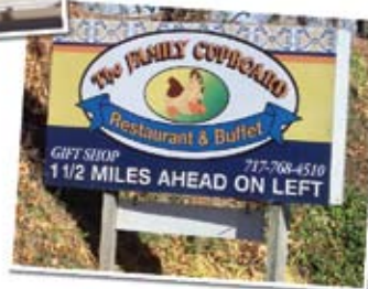
This 4' x 8', .040 thick aluminum billboard is mounted over an existing wooden frame. ▼
